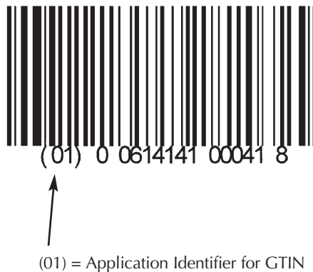
Figure 5.5 EAN/UCC-14 Encoded in a UCC/EAN-128 Bar Code Symbol
