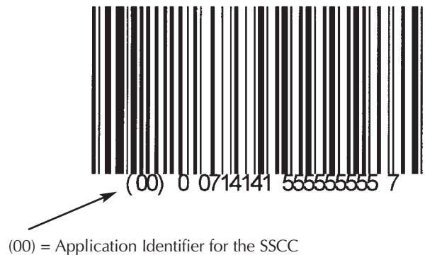
Figure 5.8 SSCC Encoded in a UCC/EAN-128 Bar Code Symbol
