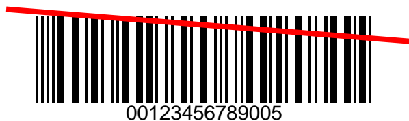
415 Figure 4-6: "From top to bottom" scan
