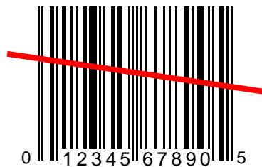
Figure 4-9: Scan not 90° to symbol bars and spaces
