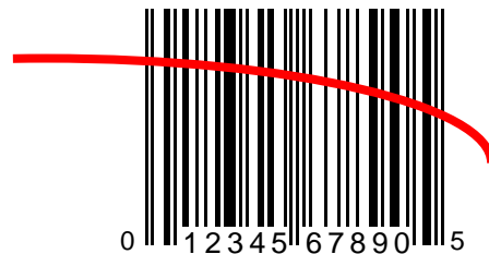
424 Figure 4-8: "Curved motion" scan
