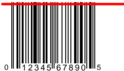
420 Figure 4-7: "Close to the top" scan
