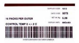
Labels printed in 'picket fence format: White lines running through the height of the bar code. Massive problem that can mean that part of the bar (or even a whole bar) is missing. Leading to failure for the ISO grades defects, decodeability and decode. See Below.
